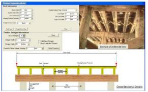
the mature capabilities required to support a deployed engineering assessment team in the expedient reconnaissance (recon) and loadcapacity determination of offload structures, providing the necessary data for planning and design of any required repairs.
